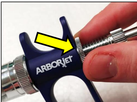
When dosage has been set, twist Stop Nut to lock in place
