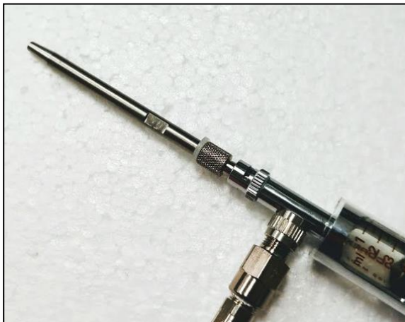
STINGER Needle modification on QUIK-JET Device
