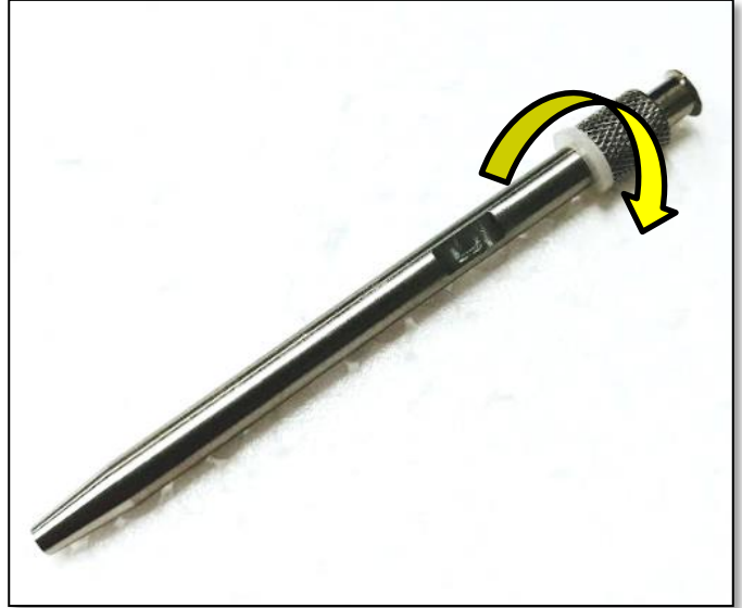
Twist Stinger Needle into Luer Fitting
