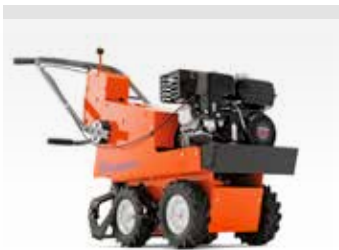
HUSQVARNA SC18 Heavy-duty five speed transmission and variable speed throttle provide increased maneuverability. Durable Honda engine and dual chain drive system mean more work time. Honda GX160 engine, 4.8 hp*. Operating width 18.0 in., operating depth variable to 2.5 in. 2 cutting speeds, 2 transport, 1 reverse.
