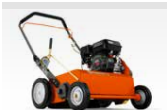
HUSQVARNA SD22 This compact, high-performance seeder makes quick work of putting down new seed. The delta blade reel cuts slits in the turf for efficient seed placement. Honda (SD22H) GX160 engine, 4.8 hp* or Briggs & Stratton 900 Series engine, 9.0 ft.-lb., gross torque*. Operating width 22 in. Seed hopper capacity 30 lbs.
