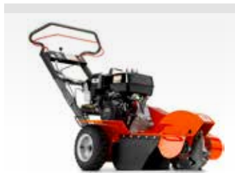
HUSQVARNA SG13 Heavy-duty greasable bearings support the 14-inch carbide cutting wheel. Compact design creates clean sight lines to your work and allows for greater maneuverability. Honda GX390 engine, 11.7 hp*. Cutting depth variable up to 12 in. with adjustable handle. 3 cutting teeth. Welded steel construction. 12 in. pneumatic tires.
