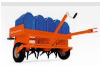
HUSQVARNA TA48 Easy to use towable aerator has the capacity to aerate up to four acres per hour. Operating width 48 in., operating depth variable to 3 in. Optional removable weights (5 gallon containers).
