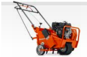
HUSQVARNA AR19 Combining ease of use and excellent handling with power and performance, these aerators are a pleasure to operate and deliver great results. Honda GX120 engine, 3.5 hp or Briggs & Stratton 900 Series engine, 9.0 ft.-lb., gross torque*. Operating width 19 in. Operating depth 3 in.
