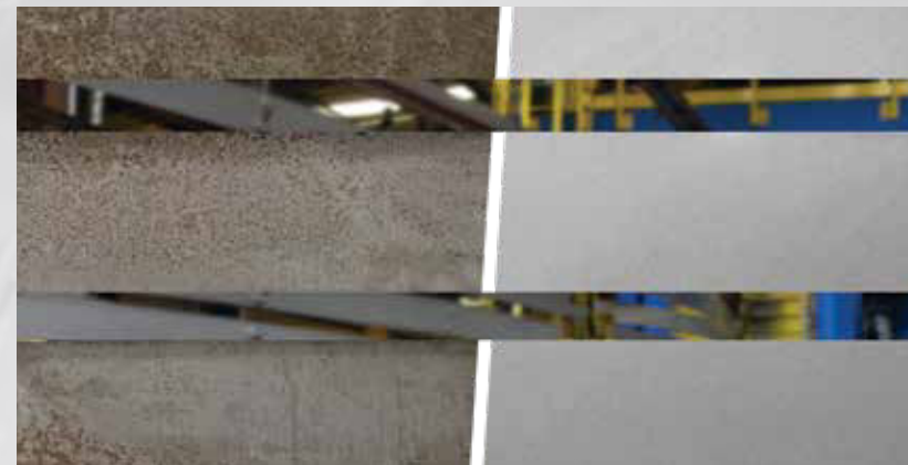
After blasting, the steel is in near white metal condition in compliance with SSPC 10/ NANCE and SSPC 5.1.4. standards.
