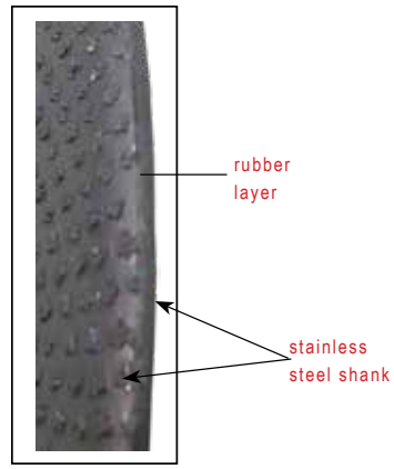
flexible sandwich construction
